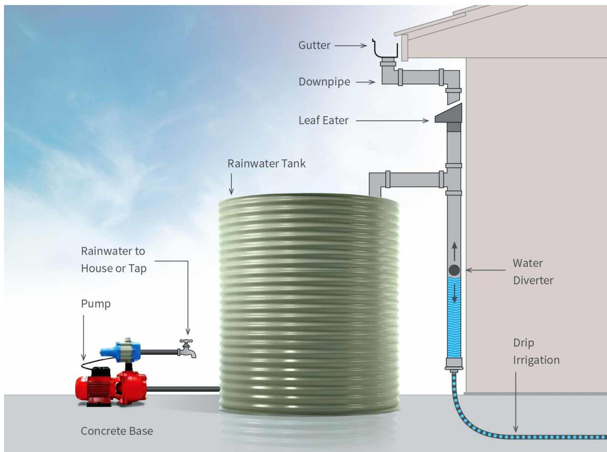
Figure 1.0 – Typical Rainwater Tank – Stratco
